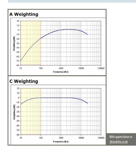
It's obvious that a C-weighted filter picks up vastly more noise (literally, exponentially more) in the low frequency and infrasound range—the yellow zone on both graphs. It's equally obvious that an A-weighted filter picks up exponentially less and less LFN and infrasound as the frequency drops. (Notice that the noise data are plotted on logarithmic graph paper. This explains why the intervals between levels of frequency are unequal. Frequency is measured in Hz = Hertz.)
